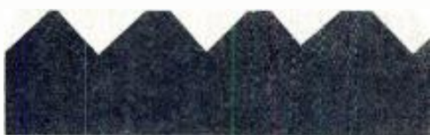
Microphotograph of grooves and cross-section of conventional two-channel stereo disc show lateral and vertical 45/45 amplitude modulation. Note that groove at right is silent, or unmodulated.
