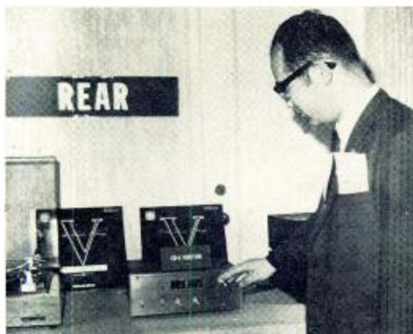
JVC's entry in the quad contest was demonstrated at last AES convention. Disc-playback adaptor includes a pair of VU meters, compatibly plays back both four- and two-channel stereo recordings.
