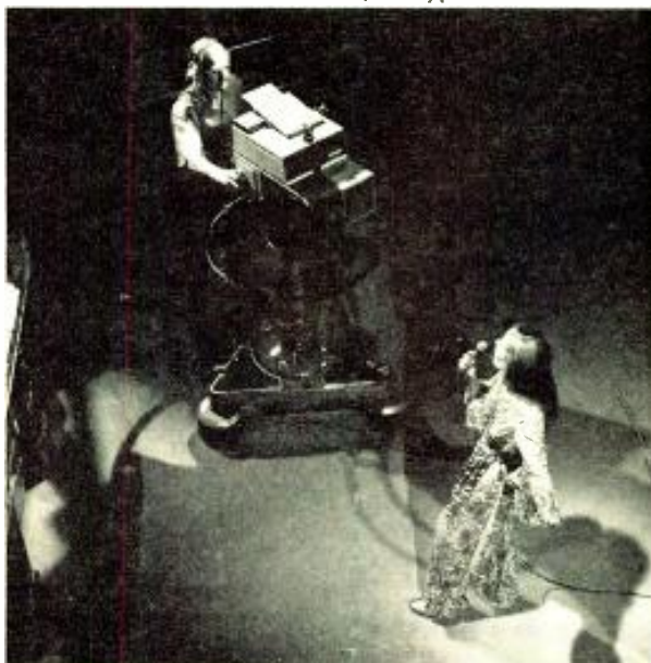
Overall length of the Mark VIII camera, including a studio zoom lens and a tiltable viewfinder, is 22¾ in.
